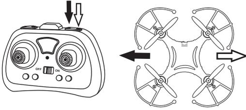
If the Quadrone leans to the right, press the L button until it straightens out.
