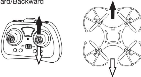
Push the directional joystick to forward. The Quadrone will fly forward.
