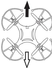
If the Quadrone leans forward, press the B button until it balances out.
