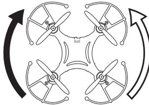
If the Quadrone turns to the right, press the L button until it straightens out.
