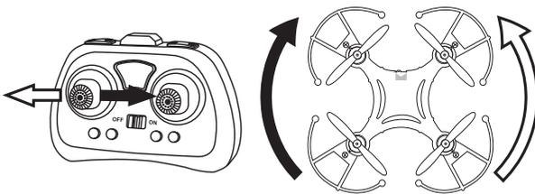
Push the throttle joystick to the right. The Quadrone will turn to right.
